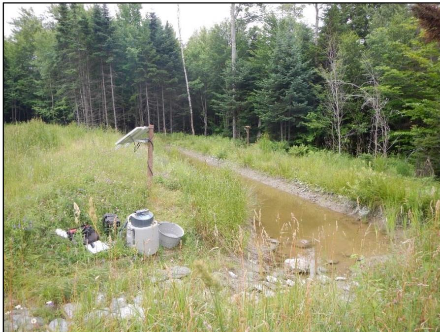
**Photograph 1. Automated sampler at LS-A9 inlet. Flow enters LS-A9 in the stone-lined swale in the foreground of the photograph (VHB, 07/08/16).**
